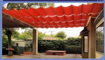
Our Pergoshade can span to a width of 5mtr and travel to a length of 18mtrs [covering area 90sqmtr.] with a single motorized drawing-system on guided cables and pulleys. The system is fixed to the opposite ends and the cables link the two ends to facilitate the travel of the flat or festooned fabric in panel widths ranging between 450 to 600mm.
